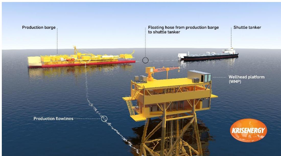
Mini Phase 1A simplifies the original Phase 1A development with a smaller platform, fewer initial development wells and the use of lower cost leased shuttle tankers versus the original plan for a permanent floating storage and offloading vessel (“FSO”).
